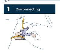
Open FoleySafe lead with its snap latch on its' ends'.
